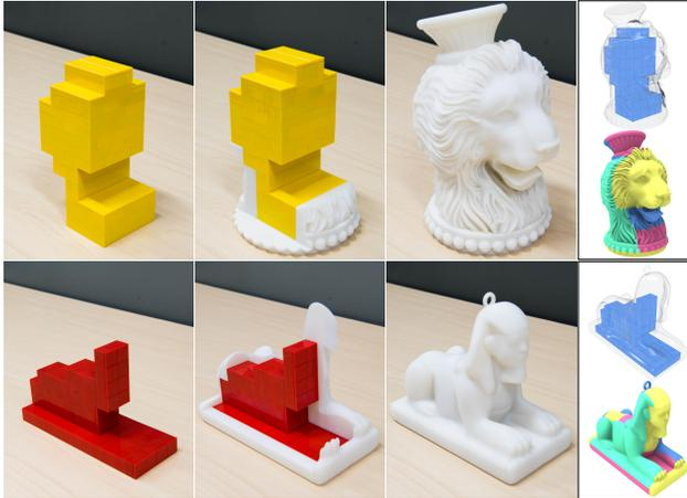
Fig. 20. Physical fabrication results with LEGO-built internal core. From left to right: internal cores built from LEGO bricks, some residual parts attached, the completed assemblies, and then the internal core and the parts composition in virtual.
