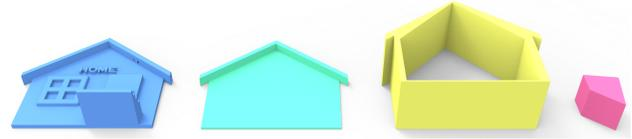
Fig. 18. The optimal pyramidal decomposition created by a participant on the House model has only four residual parts and nearly zero support waste.
